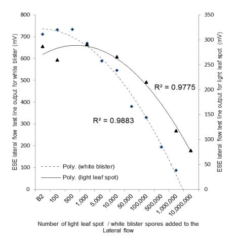
**Figure 12.** Mixed spore concentrations of *Albugo candida* (white blister) and *Pyrenopeziza* brassicae (light leaf spot) applied to multiplex (two test lines for independent measurement of mixed spore types in a sample) lateral flow devices
