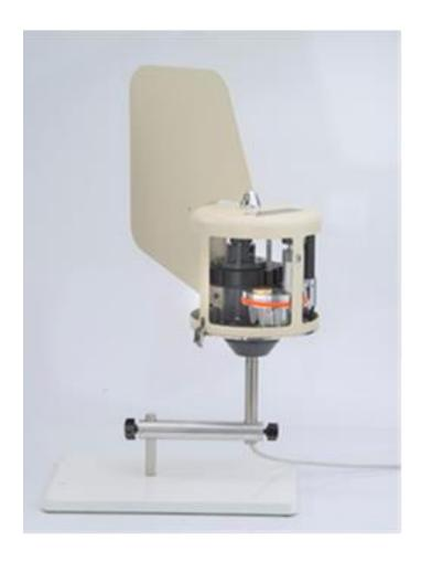
Figure 2. Automatic Multi-vial field cyclone sampler (www.burkard.co.uk)
